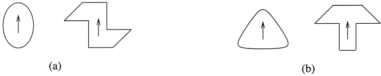
Fig. 4. (a) Particle shapes with a two-fold symmetry perpendicular to their magnetization. The arrow indicates the direction of magnetization. (b) Particle shapes lacking two-fold symmetry perpendicular to their magnetization.
